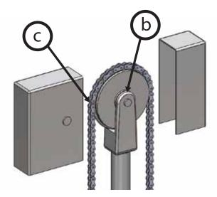
Remove screw to access the chain guide.
