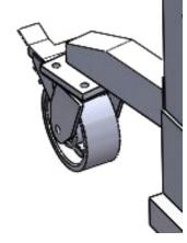
Lock shown on the Caster Wheel in the unlock position.
