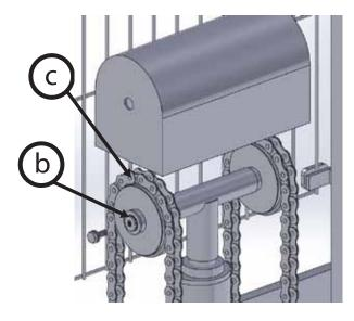
Remove screw to access the chain guide.
