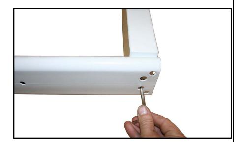
Place the stand on its feet. Attach the mid cross member to the stand with the bolts identified as " **C** " in the hardware section of this manual. Use the 6mm Hex tool for these bolts.
