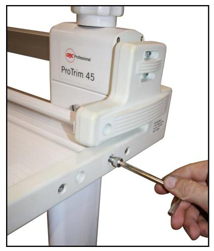
Remove the wire ties from the waste curtain, and then install the waste curtain in the rear of the trimmer as shown in the photo.
