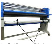
Media Alignment disks keep supply rolls from telescoping
