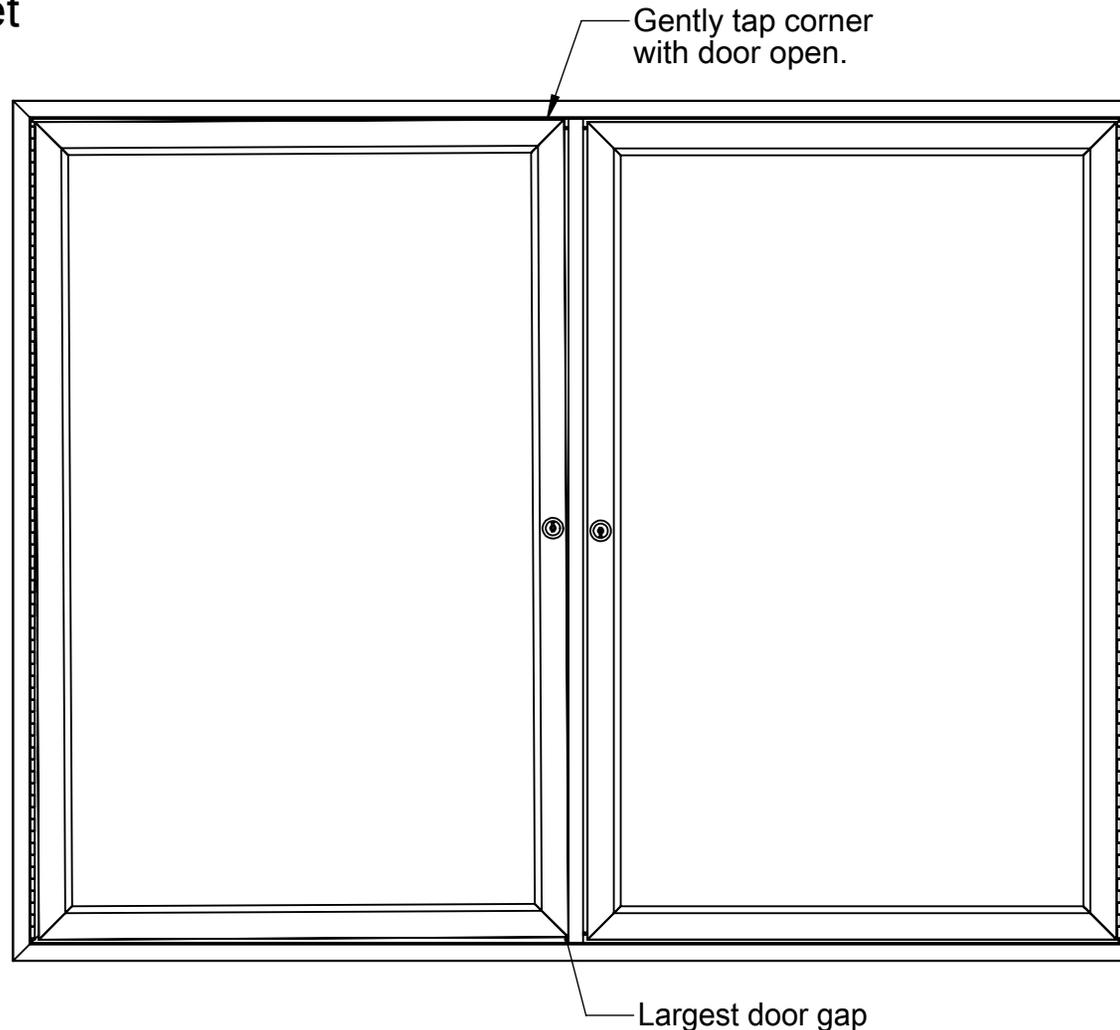
Your new Ghent Message Center has been assembled and inspected to Ghent's high quality standards. Occasionally during shipment, your message center's door(s) may shift. This shift results in an uneven gap between the door(s) and the body of your unit.
