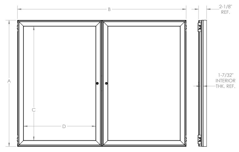
Walnut framing shall be stained first and then clear-coated. Oak framing shall be clear-coated only. Door shall be 1/8" acrylic. Door to be equippped with nickel hinges and built-in lock with keys. The back panel of the case shall be fitted with optional vinyl, cork, tackboard, Porcelain, or changeable letterpanels for interior use. Available Sizes:
