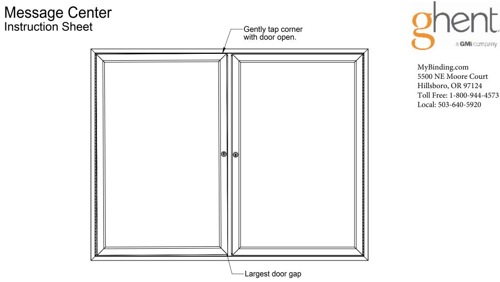
Your new Ghent Message Center has been assembled and inspected to Ghent's high quality standards. Occassionally during shipment, your message center's door(s) may shift. This shift results in an uneven gap between the door(s) and the body of your unit.
