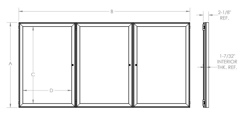
Walnut framing shall be stained first and then clear-coated. Oak framing shall be clear-coated only. Door shall be 1/8" acrylic. Door to be equippped with nickel hinges and built-in lock with keys. The back panel of the case shall be fitted with optional vinyl, cork, tackboard, Porcelain, or changeable letterpanels for interior use. Available Sizes:
