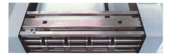
Remove the safety cover. The balance bar is the widest one now visible and has two black screws in the middle of it. Using an Allen key, adjust the depth of each side of crease. Bring it even and/or change over all depth by loosening/tightening either/or both of the black screws.
