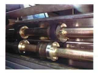
Adjust the location of the metal exit wheel and the rubber exit wheel to where the perf blade and lower knife are up against each other.
