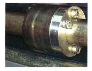
Once the lower knife is installed, loosen the rubber exit wheel with a 2mm Allen key. Use M3\*6 Allen screws to install the perf blade on the rubber exit wheel, tighten the screws with 2.5mm Allen key. In the same fashion as explained above, install the other perf blade.
