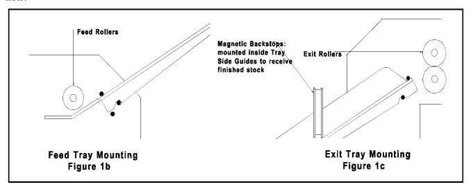
**Note:** It is critical that the operator side tray guide be moved all the way over to the operator side of the machine to ensure that the stock being processed through the machine passes directly underneath the photocell. If the stock does not pass directly underneath the photocell, the machines will not recognise sheets and the program being run will not be initiated.
