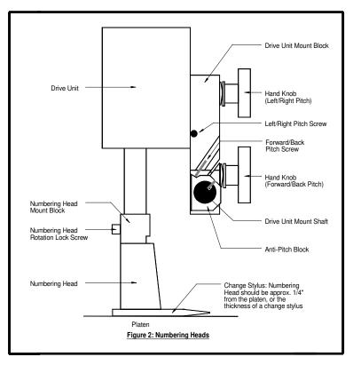
The height of the numbering head has been factory set and it is critical to the proper performance of the drive unit and numbering head. This distance is approximately 3" or the thickness of a numbering wheel change stylus. However, the numbering head must be levelled to ensure that the numbering wheels strikes the sheet square to provide a quality inked impression and a flat crash impression on carbonless sets. This will be discussed later (Section 4.11).
