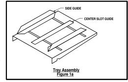
screw on the nylon wing nuts to secure the pieces on the tray. The operator side tray guide of both the feed and exit tray should be pulled all the way over to the operator side before tightening its two wing nuts.
