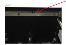
To remove the back cover: remove the screws on either side of the back cover, as well as on top. They will all be visible.
