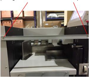
Remove the second bracket by removing and replacing the two hex key screws which secure the table extensions on top, and the two screws at the bottom.
