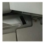
**2. front guide knob-** Turn the knob clockwise to decrease the gap (shown in illutration below) if double feeding occurs, or turn the knob counter-clockwise to increase the gap if the paper is unable to pass through.
