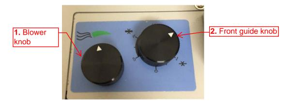
**1. blower knob-** Turn the knob clockwise to make the air vents smaller (see image underneath to left), and counter-clockwise to increase the air vent sizes (see image underneath to right). If stock is thin, the air vent size should be smaller, air vent sizes should increase as paper thickness increases. This air adjustment is important for proper feeding. If a sheet is not being picked up by the belt to feed please adjust the air.
