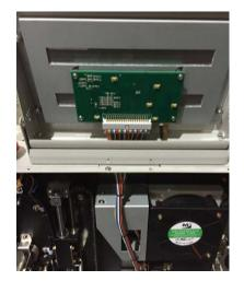
Next, Remove the back cover from the touchscreen. It will take four screws that are located on both sides.
