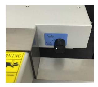
**Skew adjustment-** Using the knob shown below the user can adjust for any skew in the crease or perf of the sheet. If the wheel is turned downward the feed table will move to the left. If the wheel is moved upwards the feed table will move back right.
