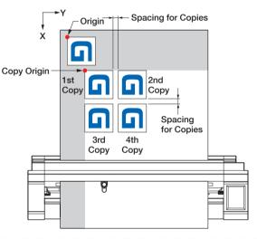
**1.** Perform the cut once with the data to copy. The cutting data will be retained in the buffer memory.
