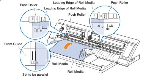
$\overline{Z}$  Align the left edge of the roll media with the "I" marking of the "  $\Box_{\mathbb{D}}$  " mark on the front guide.
