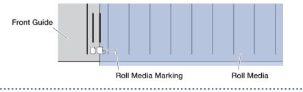
**8.** The roll media is set after detecting the width and leading edge. Operate the device by following the on-screen instructions when an error message appears.
