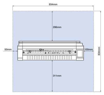
When using the roll media stocker and installing the device on a table, use a table that is leveled and solid with a top panel that is at least  $934 \times 502$  mm in size.
