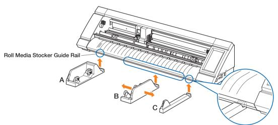
Set Part D to the groove on the edge of Part A, B, and C as shown in the figure below.
