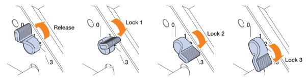
When the media lock lever was set to incorrect position, the message of correct position will be displayed. Set the media set lever - right to the correct position according with the message
