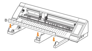
Slide the rollers toward forward when using a 2 inch media core or toward backward when using a 3 inch media core. Loosen the knob to move the roller and fasten the knob to fix the roller in place. Place the roll media on top of the rollers so that the media can be pulled out from the top.
