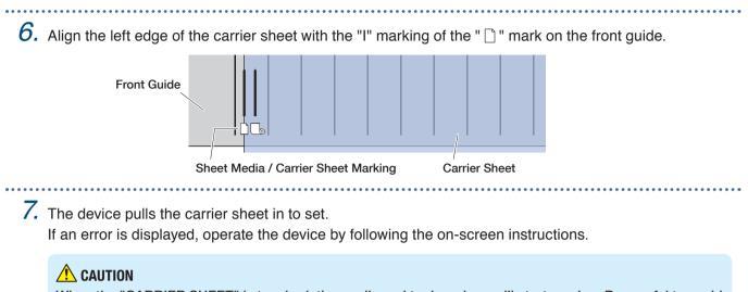
When the "CARRIER SHEET" is touched, the media and tool carriage will start moving. Be careful to avoid contact with your body or any object.
