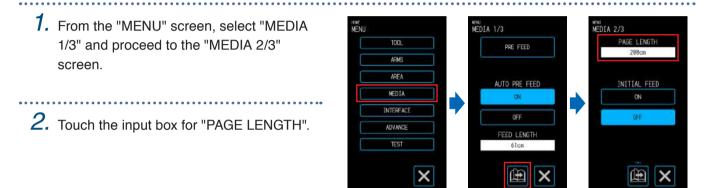
3. Input the page length and confirm the input with the  $\checkmark$  (Confirm).
