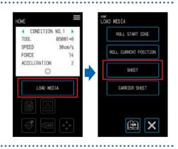
5. Evenly position the edge of the sheet media up against the push rollers. Pass the sheet media under the push roller positioning guide and load it so that it is parallel with the front guide.
