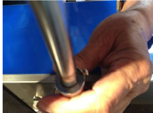
Figure 6. Ensure the groove in the long shaft matches that in the gear
