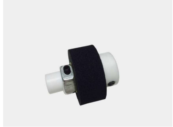
Figure 21. Ink roller installed on ink roller holder
