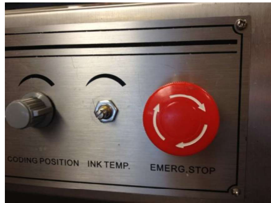
Figure 28. Remove Washer Holding Ink Temperature Potentiometer
