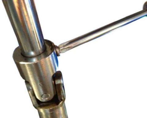
Figure 7. Screw the long shaft to the umbrella gear base.
