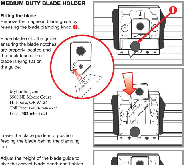
give the correct blade depth and tighten the blade clamping screw **()**.
