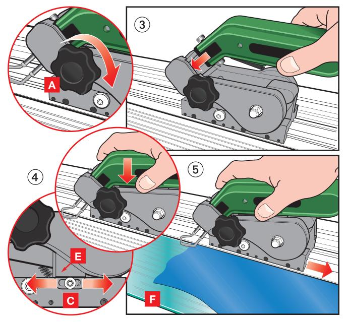
③ To fit the Hot Knife, simply insert it into the holder ensuring the nose of the Hot Knife is seated fully into its recess.
