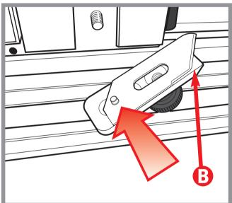
Before tightening the clamping screw the blade depth can be adjusted by sliding the adjustment knob up or down to retract or extend the blade. It is good practice to set the depth so that the minimum amount of blade is exposed to just cut through the material, it takes much less effort and produces a better cut.
