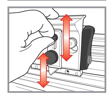
The VA (vertical action) cutting head holds two cutters which can be changed and used independently of each other. Each of the standard GRAPHIK blade holders can be set to cut at different depths and in either direction by simply adjusting or flipping the blade over in the holder. You can also push or pull the cutting head to suit your own comfort.
