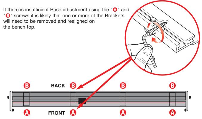
Place two of the long wood screws "A" in the front holes of the Fixed Arms and partially insert them into the bench surface but do not tighten. Loosen, by one full turn anti-clockwise, the four hexagon socket screws "B" joining the Fixed Arms to the Base. Fully insert the two wood screws "A".
