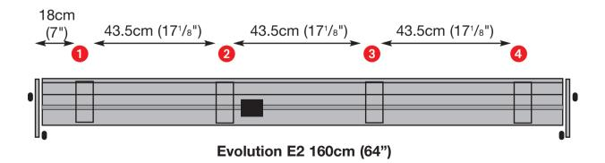
Lift the Evolution E2 cutter bar from its crate **but do not remove the clear plastic stretch-wrap bands** holding the base to the cutter bar. Place the Evolution E2 centrally on the Brackets and manoeuvre it until the base is located properly down on each of the Brackets.
