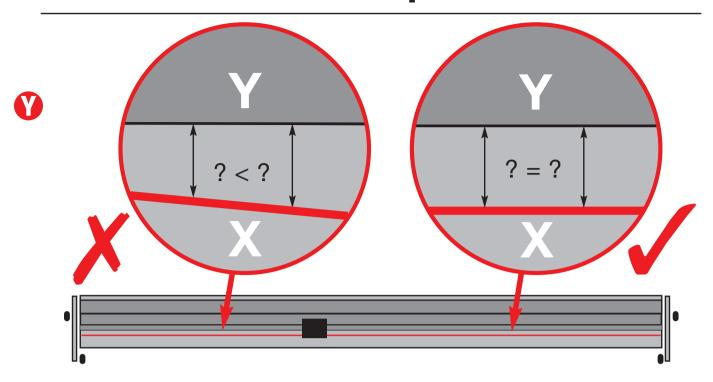
**Adjust** the straightness of the Base by adjusting the front "A" and rear "B" grub screws in the Base Fixing Brackets:
