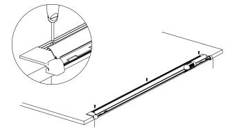
Fix a piece of 3mm MDF, PVC foamboard, or similar material to the table top as shown to bring the table surface in line with the base plate level of the Cutter.
