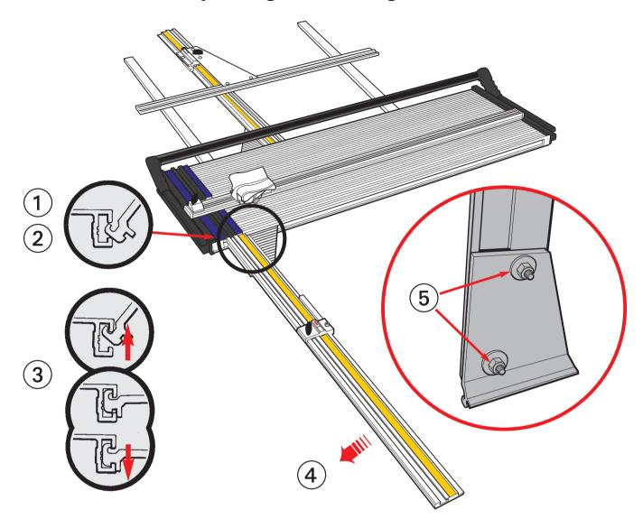
The Squaring Arm is used to cut materials precisely square and to a pre-determined size. Before fitting, check that the End Plate is square by carrying out the test on the 'Maintenance – Squaring' page 4.1, adjust if necessary
