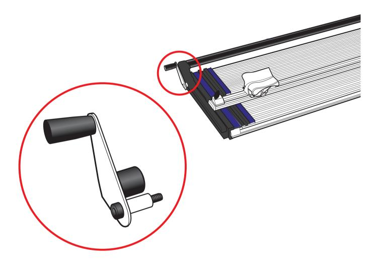
The Lift and Hold is used to raise and hold the Cutterbar above the base so you can have both hands free when positioning the material ready for cutting.
