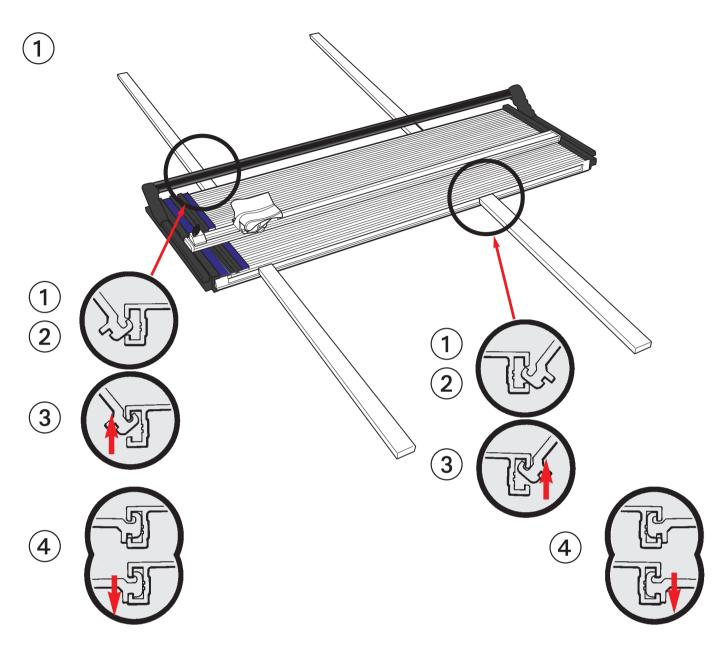
The Base Extension Arms are packed in pairs and can be fitted to either side of the Base. When large boards are cut on the machine they give the support necessary to keep the material flat for accurate cutting.
