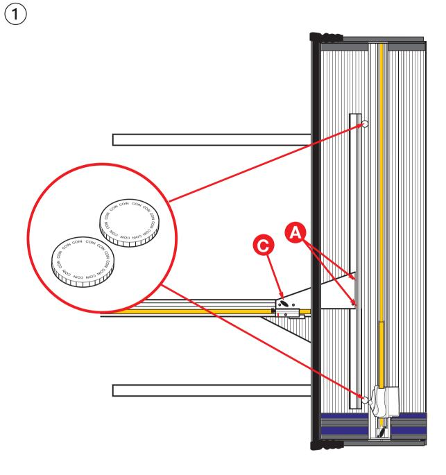
■ THE ALIGNMENT OF THE CUTTING FENCE T-Bar with the Cutterbar is checked using two identical coins.
