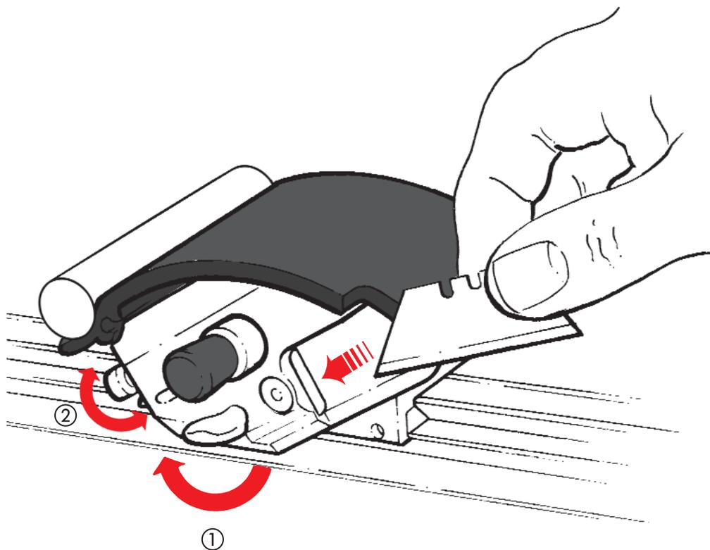
**Inserting and setting the blade**
