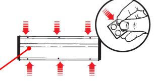
Rubber feet to be equally spaced along left and right edges of the base.
