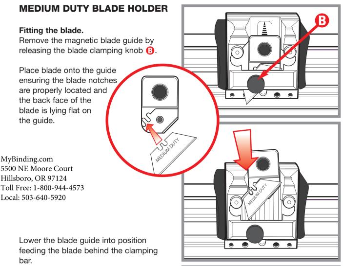
Adjust the height of the blade guide to give the correct blade depth and tighten the blade clamping screw **B**.
