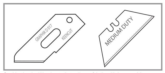
Consideration should be given to the toughness of the board being cut and the maximum depth of cut. It is recommended that heavy materials such as PVC foamboard should ideally be cut using the Graphik blade holder and to a maximum of 6mm (0.25") whereas, lighter materials like foam centred board can be cut up to the maximum cutting depth of the blade being used.
