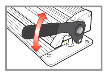
Lifting vertically remove the cutter from both guide rods at the same time. Check that the Base Plate is laying flat on the table surface along its length. If necessary use paper or card under the full width of the Integra base to make it level on a bench top that is not flat.
