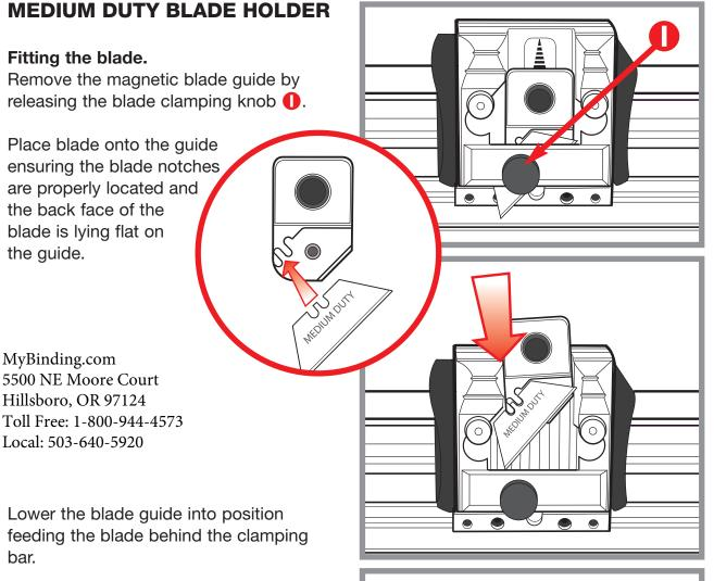
Adjust the height of the blade guide to give the correct blade depth and tighten the blade clamping screw **()**.
