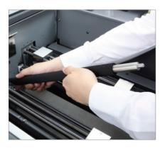
**EASY MAINTENANCE** The Velocity now has detachable rollers, not only making cleaning easy, but gives better access to components in case of a paper jam.
