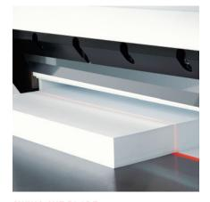
SWING CUT BLADE The German high speed steel blade with swing cut movement provides the highest level of cutting accuracy.
