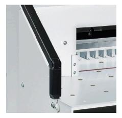
**IR SAFETY CURTAIN** The IR light beam safety curtain covers the work area to ensure the highest level of operator safety.
