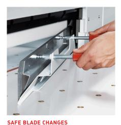
Blade changes can be made without removing the machine covers. The handy blade changing device covers the cutting edge of blade.
