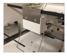
**BELT FEED SYSTEM** A belt fed, air suction system allows trouble-free feeding of coated stock.
