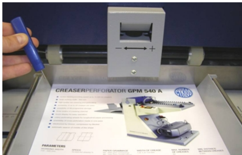
Fig. 11: Adjusting the feeding wheels (position 29) with the Allen "T" key
