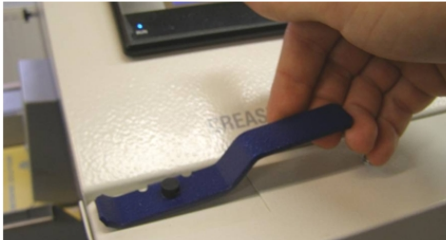
Fig. 17: Pulling callipers to the upper position
