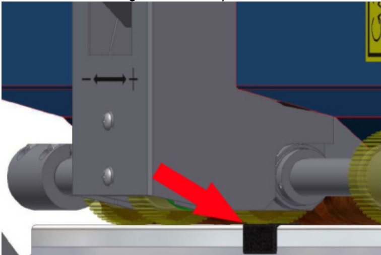
Fig. 34: The gap between feeding wheel and separator must be 0.002" – 0.004" wide.
