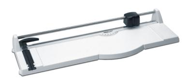
Ergonomic safety cutting head with fully enclosed, hardened steel rotary blade. Transparent bar clamp with automatic clamping action. Extendable bracket with measurement scale can be used as a front or back gauge. Protractor with alignment indicators on clamp bar and cutting table for angle cuts. Dual measurement scales on cutting table. Constructed of sturdy, impact-resistant ABS plastic with non-slip rubber feet.
