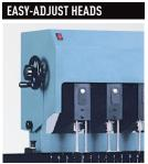
The drilling heads are easily adjustable with the calibrated hand cranks.
