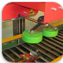
Top Flap Compression Roller to Keep Box Top Closed
