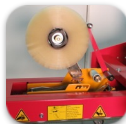
Piranha Tape Heads with Optimizer Arm
