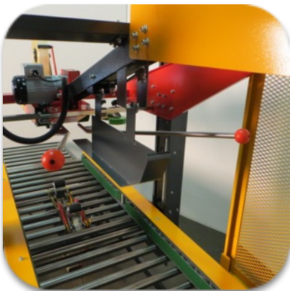
Automatic Box Folding of Major and Minor Top Flaps
