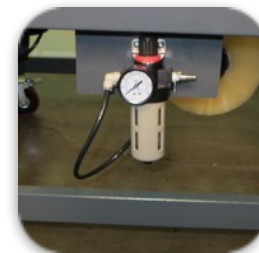
Air Required for Pneumatic Minor Flap Closer
