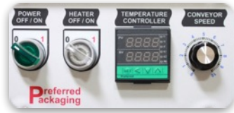
Tunnel Control Panel
