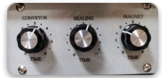
Sealer Control Panel
