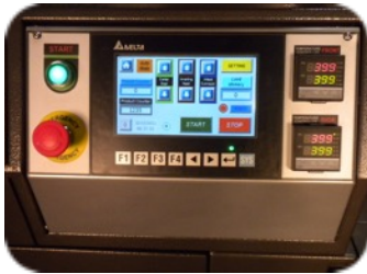
Delta PLC with 40 program memory and self-diagnostics
