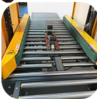
Heavy Duty Dual Side Drive Belts Move Inward to Automatically Center Box
