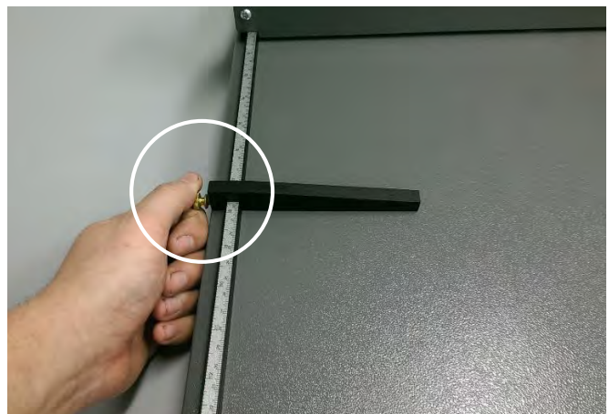
FIG 2: Position Stops, Tighten Thumbscrews
