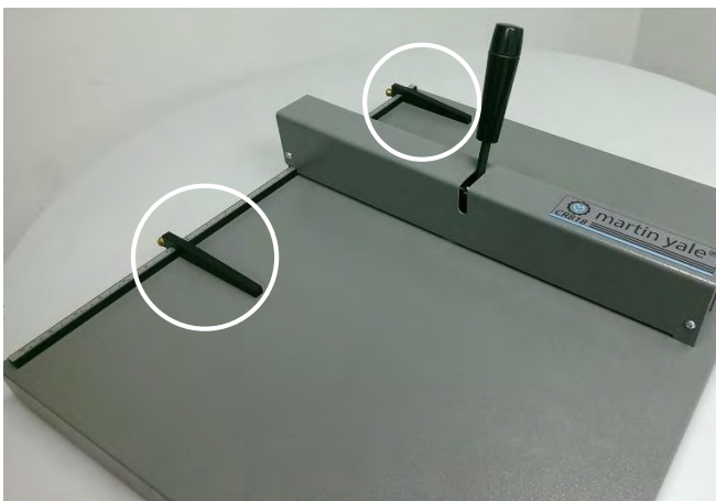
FIG 1: Install Paper Stops, Handle Upright
