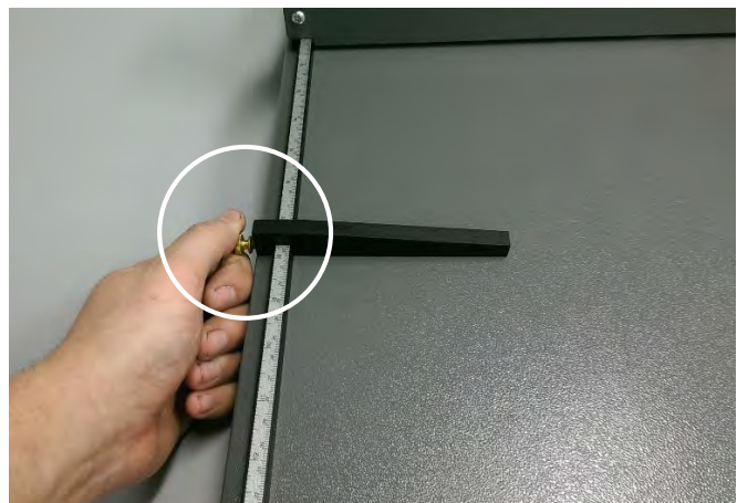
FIG 2: Position Stops, Tighten Thumbscrews
