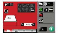
Using the screen is simplicity itself. Key in the sheet length (popular sizes are pre-set), touch the fold type for the finished product (letter, gate etc) and press the green button. The AutoCreaser Pro 50 will automatically calculate
