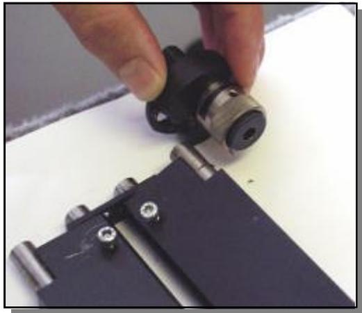
3. Using a 6mm allen key, loosen the socket head screws located inside the blade adjustment cams. Remove the screws and the blade adjustment cams.
