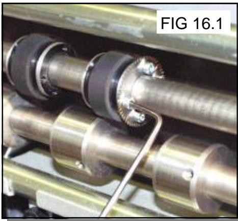
6. Using the 2.5mm allen key (supplied), take one of the matching pairs and mount on to the drive wheel. Do not secure the blade.
