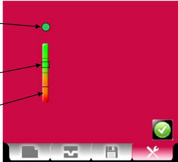
The vertical indicator scale is divided into four sections, the position of the slider indicates the strength of the beam. The strength of the beam is at its strongest towards the top half of the indicator scale (green) and at its weakest towards the bottom half of the indicator scale (red). Note the position of the slider on the indicator scale and then clean the sensors as described on Page 46.
