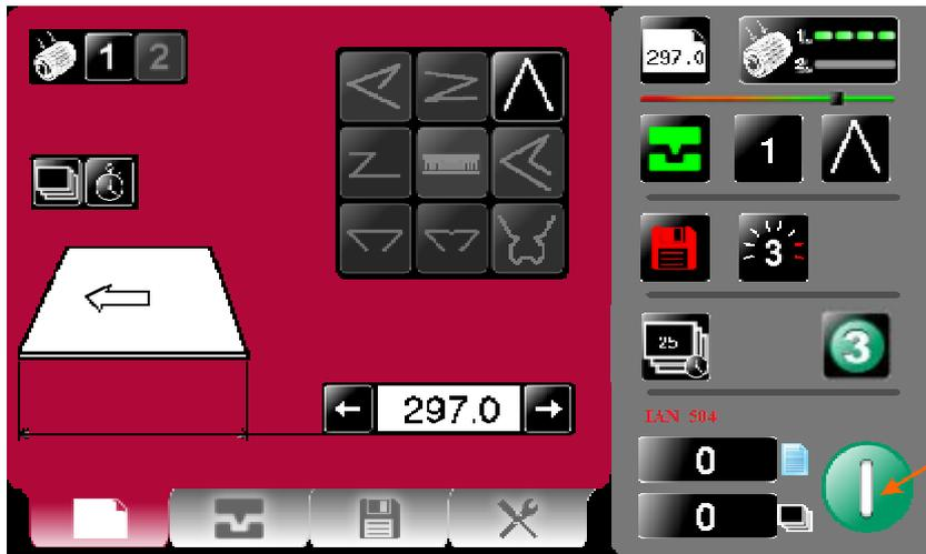
Click to start machine with settings currently shown - you will receive a notification if system switch is not on. Press again to stop Job
