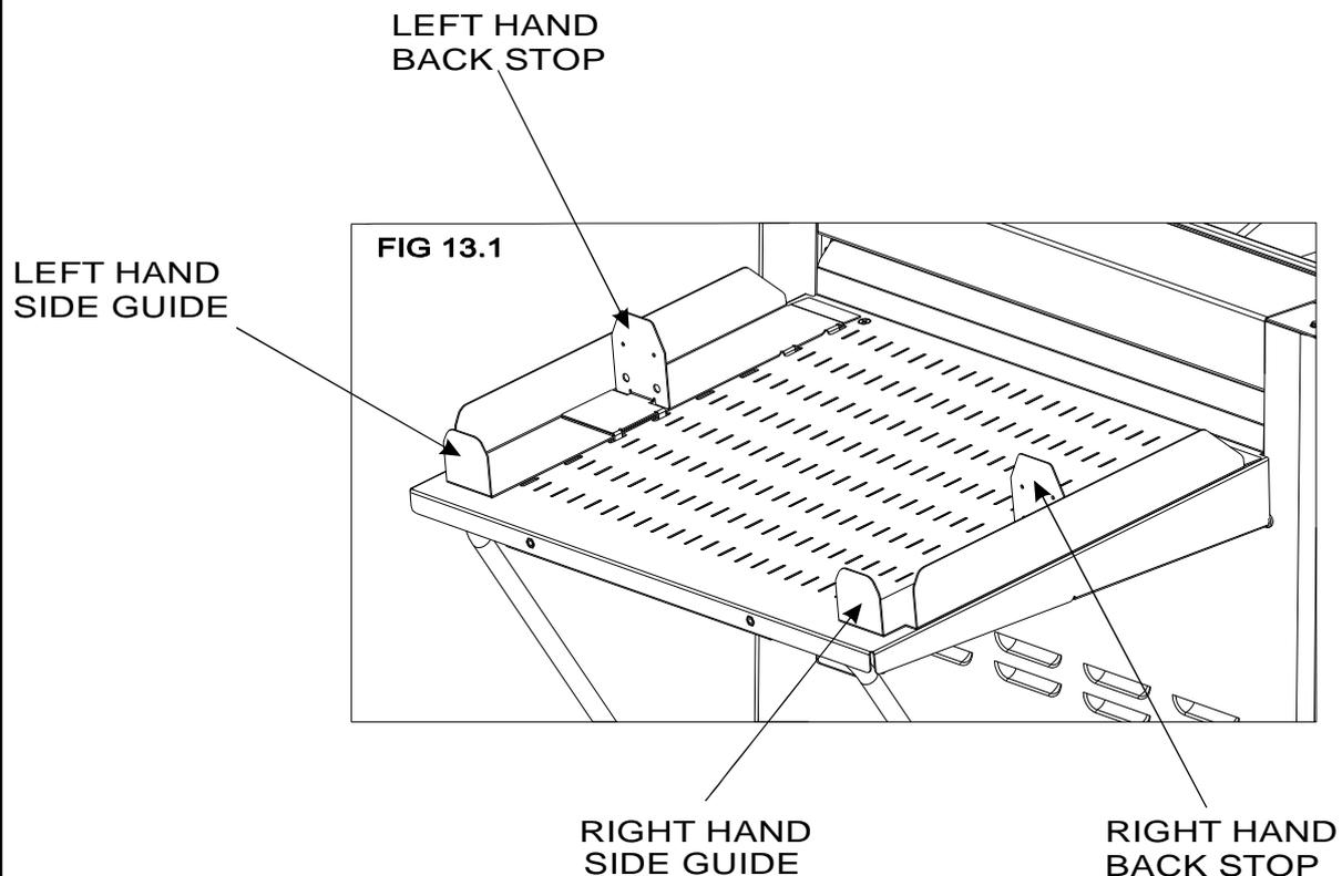
4. Whilst the sheet is between the two guides on the stacker bed, set the distance between the top of the sheet and the backstop flanges to approximately 5mm.
