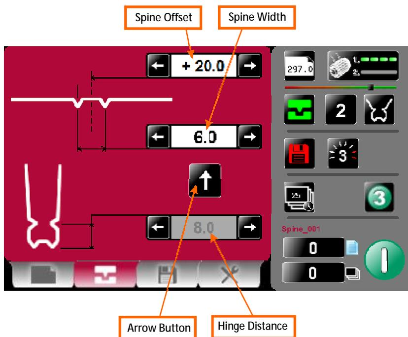
4. Enter the Spine Width dimension. If necessary, adjust the Spine Offset from the centre of the sheet.
