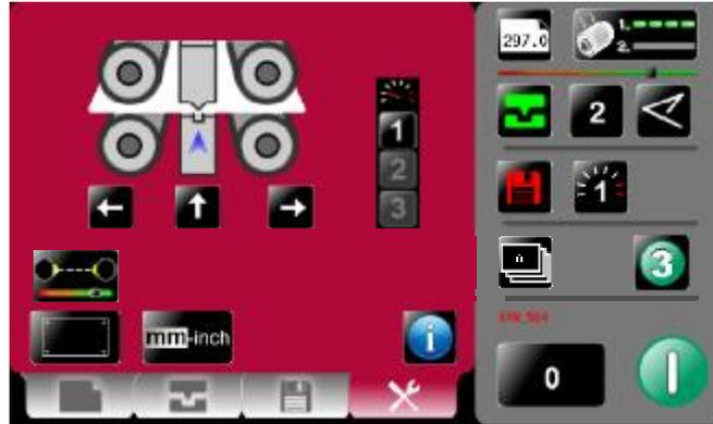
3. Press the system switch down and then select the left arrow on the touch screen, to rotate the rollers in short pulses until the sheet is gripped in the infeed rollers..
