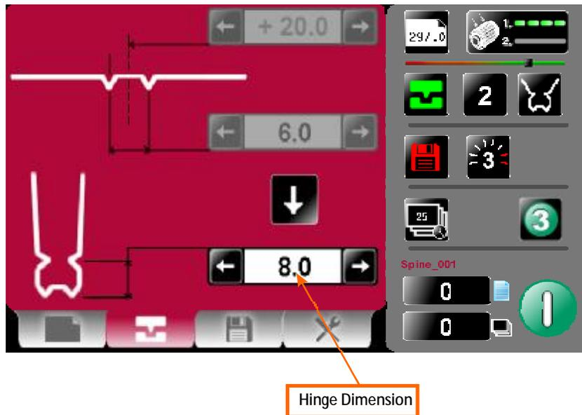
7. Select the arrow button to highlight the Spine Offset and the Spine Width dimensions.
