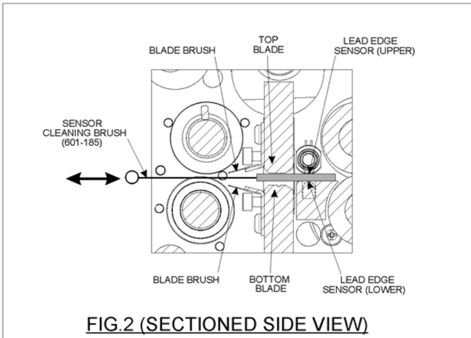
**FIG.2 (SECTIONED SIDE VIEW)**
