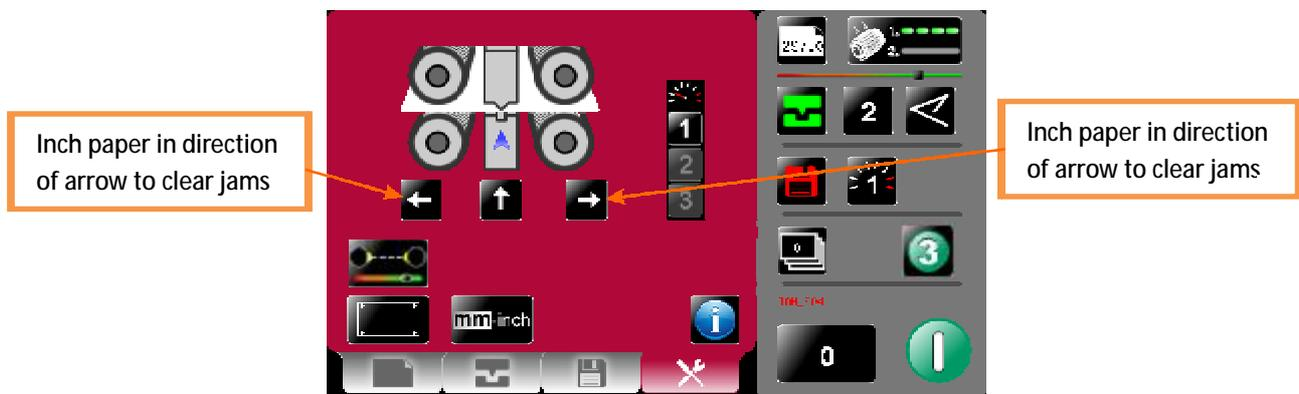
Press the system switch down and then select the right or left arrows, to rotate the rollers in short pulses.
