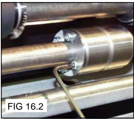
9. Using the 2mm allen key, loosen the drive hub nearest the perforating drive. Slide the drive hub away from any obstructing drive wheels or hubs in order to mount the anvils.
