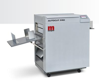
The AutoCut also has a double-feed detection sensor to avoid wasting valuable prints. In addition, it's cut-mark sensor reads any image drift and will register to ensure a consistent finish on every sheet. There is also an adjustment to allow for printed sheets that are skewed. By linking the AutoCut to the Morgana AutoFold Pro you can crease and fold in one pass, shown below.
