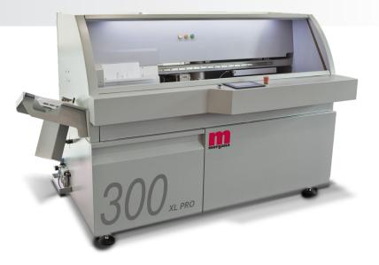
application system which is covered by no less than seven international patents. The application is direct and hermetically sealed, without odour or toxic fume emissions, and does not require extraction fans. It is possible to set different temperatures for the glue melting tank and the applicator giving greater flexibility and glue life. Another feature of this applicator is it can be cleaned and sealed automatically from the touch screen allowing for minimum glue wastage.
