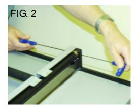
4. Depress the handle to the stop position as shown in FIG. 3, insert a 2.5mm allen key into the bronze bearing adjustment hole and rotate downwards until it stops. Repeat both sides and then tighten the four locking grub screws.
