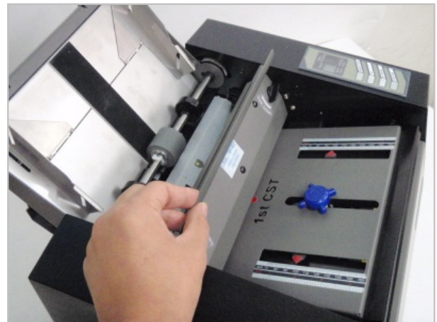
[Open the top cover by un-locking the locking knob.]
