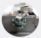
2. Adjust side guide for package size and bag width
