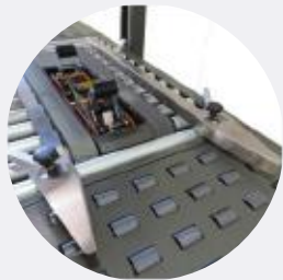
Heavy Duty Top and Bottom 4 Drive Belt System for Positive Grip Pressure
