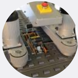
Heavy Duty Side Drive Belts for Positive Grip Pressure
