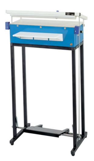
Update 07/13/16. Do not reproduce without permission. **YC-Foot Sealers** feature a sliding cutter and U-shaped sealing bar – an ideal sealer for poly tubing. The sealers are available in 18" and 24" with a cutting length of 15" and 21", respectively. The seal width is 3mm. The unit is equipped with a rectangular steel frame stand. The manufacturers replacement kit includes two elements and a knife.
