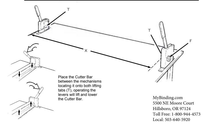
As stated before, it is important to ensure the table surface in the area between the Lift & Hold Mechanisms is flat, **particularly when cutting thin films and paper**. If the table is not flat thin materials can deflect as the blade passes resulting in a curved cut, it is wise to repeat the 'paper test' at this stage.
