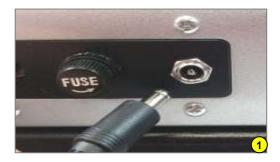
1. Plug the male connector into the receptacle at the back of the machine then connect the power cord into an electrical outlet.
