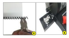
8. Use the handheld coil crimper pliers to crimp the ends to keep the document from unbinding. TIP: Periodically empty the waste bin to help ensure uninterrupted use (see figure 9).
