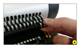
4. Disengage pins that would punch off the edge of the document by pulling them towards you. TIP: Punch a few test sheets first in order to get the proper alignment.
