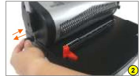
2. Adjust depth margin control from 2.5mm to 6.5mm. This controls how far or how close you want the holes to be in relation to the edge of the document.
