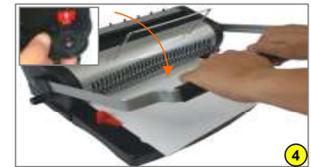
4. Adjust wire closer control to "punch" (see inset) then grasp the punch handle with 1 or 2 hands and pull down to punch holes on the document.
