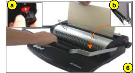
6. Adjust wire closer control to the appropriate size (see inset "a"). Insert the document into the wire closer with the wire facing downward (see inset "b") then pull the handle down to close. Remove the bound document and flip over the back cover to complete the binding process.
